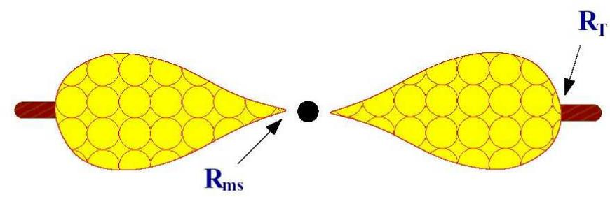
$$I_{\text{corona}} \propto R_{\text{ms}}^{-1}/R_{\text{T}} \quad I_{\text{disk}} \propto R_{\text{T}}^{-1}/R_{\text{T}} = R_{\text{T}}^{-2}$$
