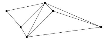
The rigidity is reflected by the fact that while each particle can move, and therefore change the position vectors, all the distances  $|\vec{r}_k - \vec{r}_\ell|$  are constant. Only the orientation and overall location can change; there is no flexing or twisting:
